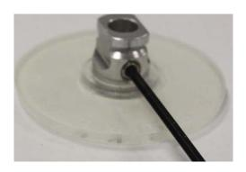
Note: if you have the newer knobs, you have to remove the socket screw before you pry off the knob.
